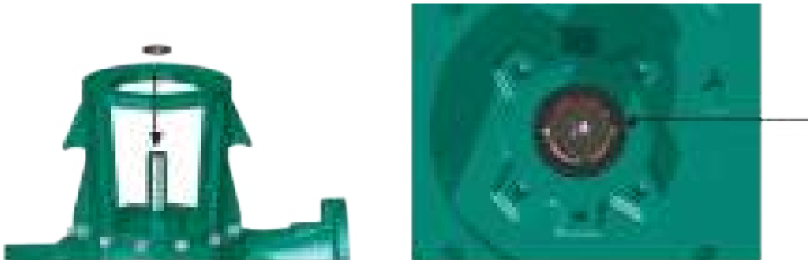
Figure 6.38 Assembling and inserting the lantern ring into the shaft until it touches the packing.
