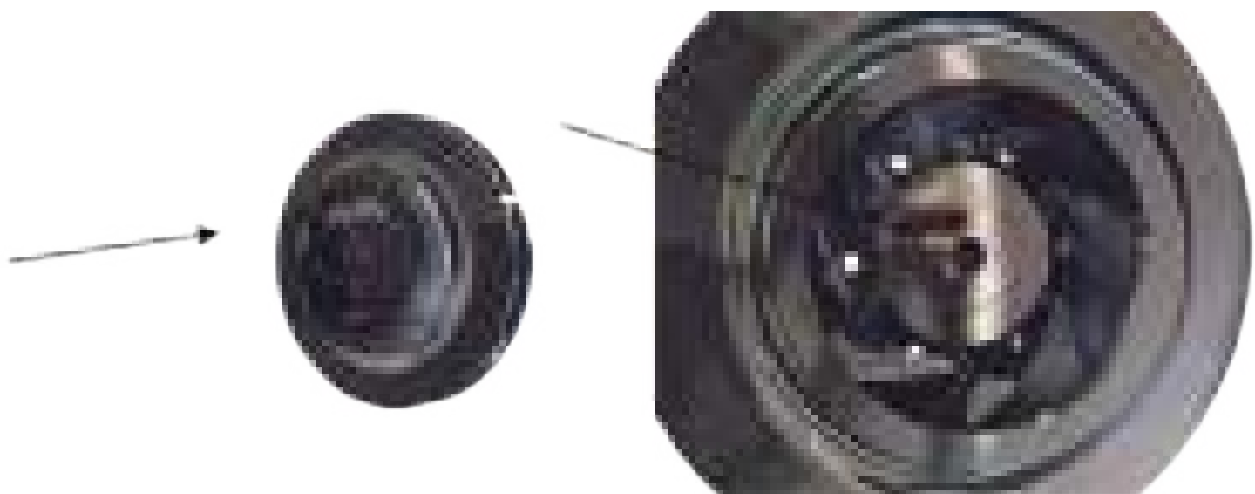
Figure 6.4 Placing the impeller lockwasher into the shaft's impeller side.
