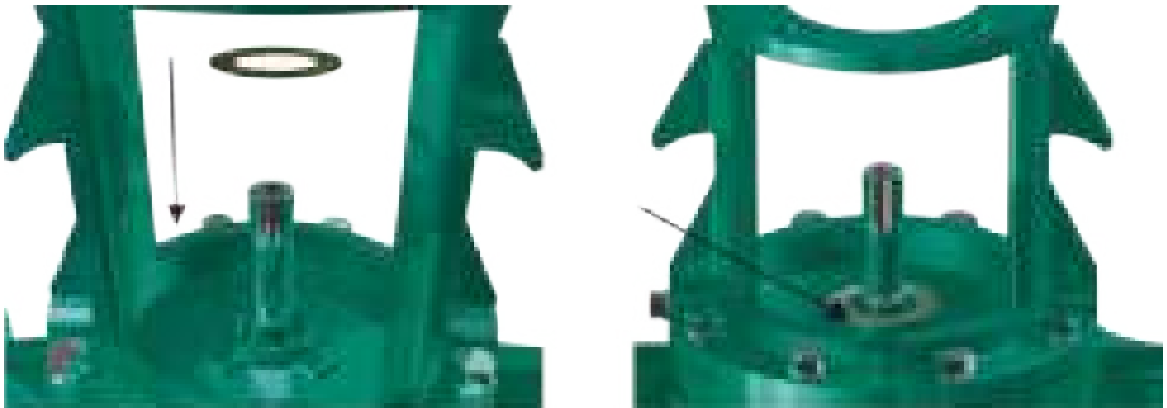
Figure 6.12 Inserting the gasket of the mechanical seal into the shaft.
