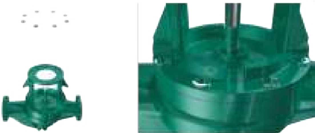
Figure 6.10 Placing the corresponding washers on the adapter matching the screwholes.
