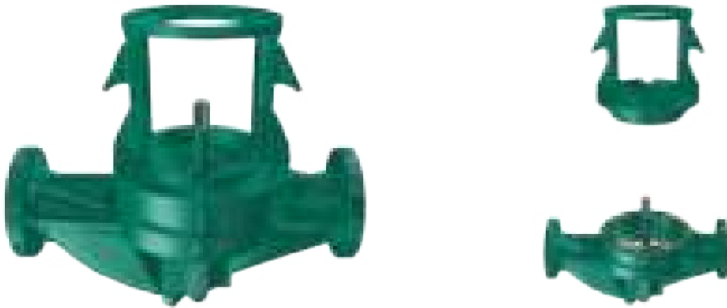
Figure 6.9 Positioning the adapter in the casing.
